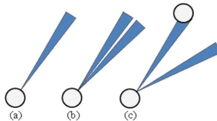
**Fig. 3** Search for a leader: (a) the search is initiated in the angle provided by the LFU, b) the search arc is expanded in left and right directions along the horizontal axis if no robot is detected in the initial region, and c) the search arc is expanded incrementally until a robot is found
