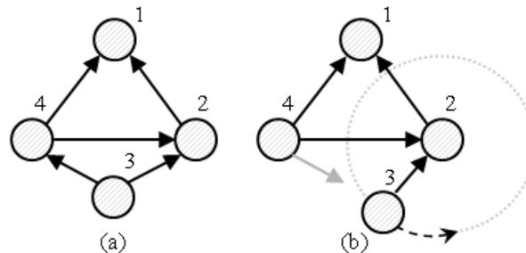
**Fig. 1** Persistent and non-persistent graphs: (a) is persistent as all vertices can maintain their relative distance during any motion, and (b) is non-persistent as vertex 4 is unable to satisfy all its distance constraints when vertex 3 moves along the dotted circle
