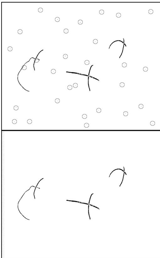
**Fig 2.**Top: A raw motion capture image with illuminated line segment based markers and noise (encircled).
