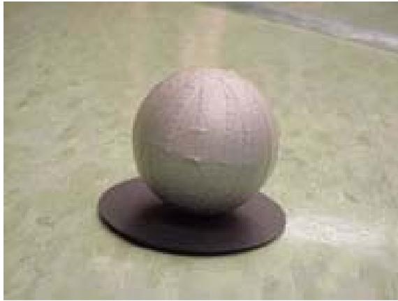
**Fig. 1** A standard spherical marker [8]. Reflects light projects light reflected from light sources.
