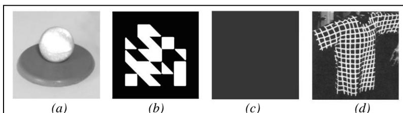
Fig. 2. (a) Passive spherical retro-reflective marker; (b) Active square marker with surface pattern [6]; (c) Active square marker with a single color painted onto its surface [7]; and (d) Active retro reflective mesh marker [8].
