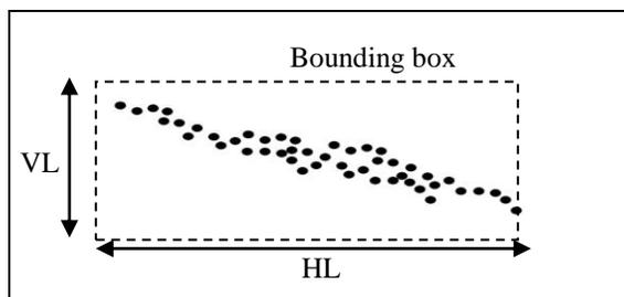
Fig. 7. Bounding box, where  $VL < HL$ , defining the line as horizontal. VL is the vertical length and HL is the horizontal length of the bounding box.
