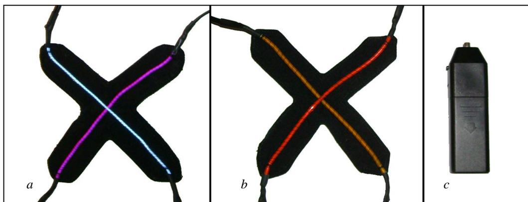
Fig. 3. Two MIC markers and a battery driven inverter. Image *a* shows a purple and turquoise MIC marker, image *b* shows a red and orange MIC marker, and image *c* shows a battery driven inverter.
