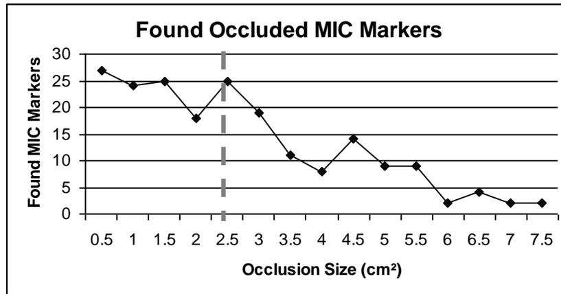
Fig. 17 Correctly found *MIC markers* as the size of occlusions increases.
