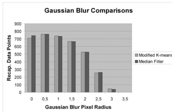
**Fig. 13.** Number of recaptured data points after images with noise and varying levels of Gaussian blur have been cleaned.
