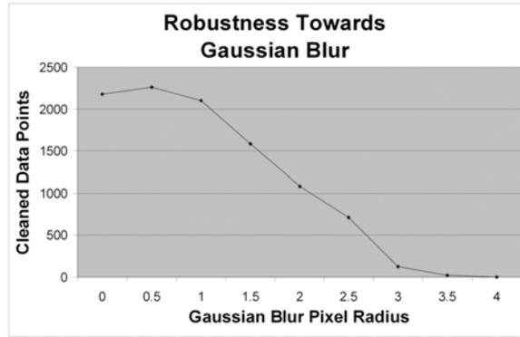
**Fig. 10.** Cleaned data points recaptured after the removal of Gaussian blur noise with varying radii using the Modified K-means.
