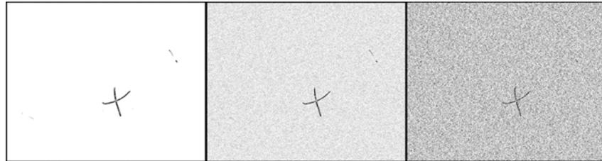
**Fig. 7.** Images with Illuminated Contour-Based Markers and Spike noise of 0, 8 and 16%.
