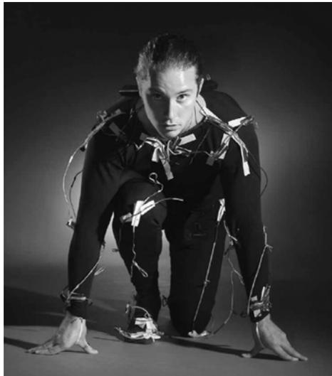
**Fig. 4.** A prototype of the bodysuit with Illuminated Contour-Based Markers attached.
