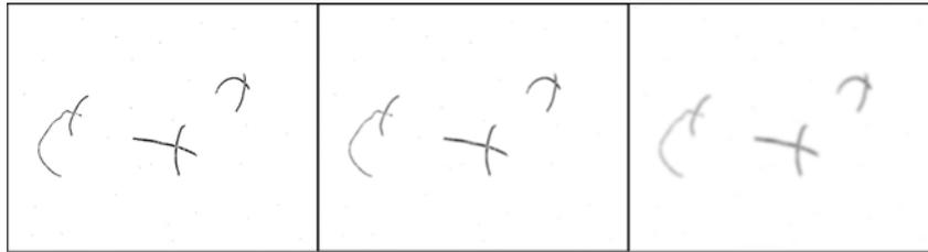
**Fig. 9.** Flattened images with Gaussian blur of 0, 2 and 4 pixels in radius before noise is removed.
